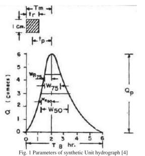
Synthetic unit graph parameters are computed using
