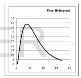
Fig. 8 Flood hydrograph for sub watershed 2 using GIUH
