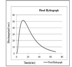
Fig. 7 Flood hydrograph for sub watershed 1 using GIUH
