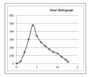
Fig. 4 Flood hydrograph for sub watershed 1 using SUH
