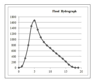
Fig. 6 Flood hydrograph for sub watershed 3 using SUH
