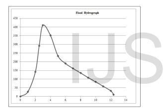
Fig. 5 Flood hydrograph for sub watershed 2 using SUH
